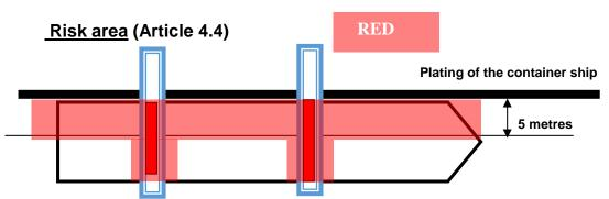
The area within five metres of the plating of the container ship without a container crane above it and/or the area in which a container crane is active.
