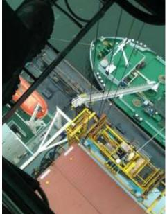
In practice, it is possible that during the use of the cradle near the connection point for the bunker boom, the cradle and the bunker boom can make contact. This risk is shown in the photographs above.
